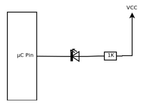
The simplest hardware is a LED connected to one pin. The following sequence initializes the pin and turns the LED on:
